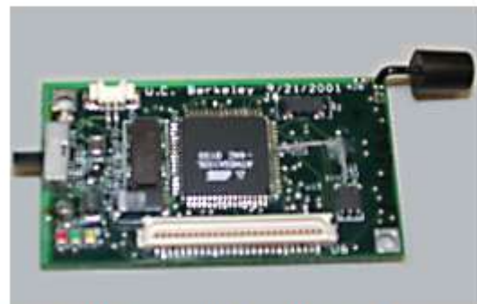
Fig. 2 The Mote with a radio antennae soldered on.
